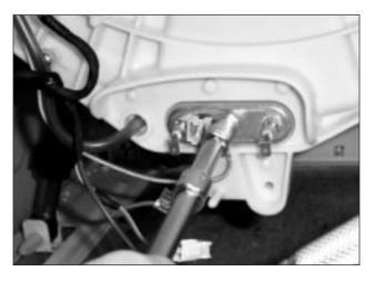
4) Loose the nut of the HEATER and pull out the HEATER.
