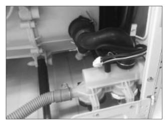
4) Remove the drain hose and the hose water supply.
