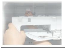
Separate the connection socket connected to the top of the Freezer and separate the ice machine from the Freezer.
