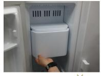
Pull the ice shaver to the front, lifting its bottom a little, to separate it.
