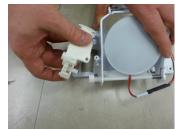
Pull out and separate the Ice Shutter inserted in the Rotation Axis of the Flap Lever.
