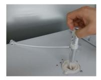
Push up the watersupplying pipe out of the top of the Freezer and pull off the water supplying pipe at the top of the refrigerator.
