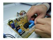
Pull the connection sockets off the Main PCB.
