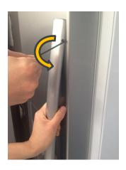
Insert allen wrench into the groove and turn it to the direction of the arrow to unfasten the bolt
