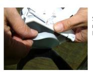
Separate the silicon rubber of the Flap Lever.
