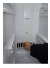
Separate the lower part of the Louver F B from the Louver F B, holding it and pulling it toward the front.
