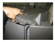
Open the Door and disassemble the Hinge Cover, lifting it from the back of it.
