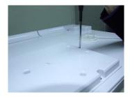
Separate the fixing bolts (4ea).
