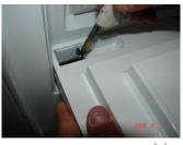
Insert the (-)Driver to the Shaft Head and pull it, holding the Home-bar Door with one hand.
