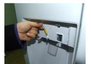
Pull out the water hose from the fixture of the I/SHUT BOX.
