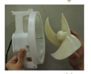
Separate the Fan blades from the C-Fan Motor Shaft.
