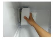
Draw the Damper cover obliquely (to the direction of the arm) to separate it from the refrigerator.
