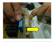
Press the temporary Hook to the rear panel (to the direction of the arrow) and separate the Main PCB board, and pull it to the rear panel (to the direction of the arrow) to take off the Main PCB.
