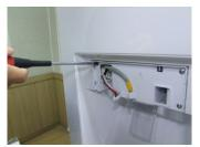
Unwind the fixing bolts (4ea) of the Dispenser Section I/SHUT BOX.
