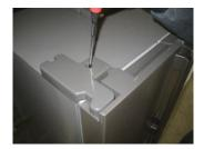
Disassemble the fixing bolts(2ea) of the Hinge Cover.
