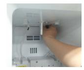
Separate the two connection sockets connected to the Geared-Motor Box at the top of the Freezer.
