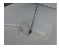
Unwind the bolt of water-supplying pipe cover at the top of the refrigerator and separate the cover from the water-supplying outlet (silicon rubber).
