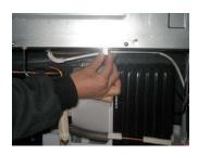
Separate the C-Fan Motor connection socket at the top to the right side of the machine room.
