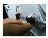
Separate the sockets (2ea) connected to the microswitch attached to the I/SHUT BOX, and pull the harness off the harness holder.
