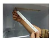
Separate the connection socket of the LED board and replace the LED.
