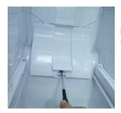
Unwind the fixing bolt (1ea) of the return cover.
