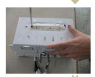
After separating the LED cover, unwind the fixing bolts (2ea) on the LED board.
