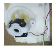
Unwind the fixing bolts(4ea) of the Motor fixing holes.
