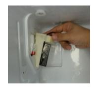
Separate the Damper from the Freezer.
