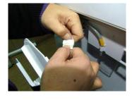
Separate the socket connected to the FCB.
