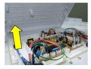
Separate the Main PCB Cover by pushing it to the Door (to the direction of the arrow).
