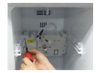
Unwind the fixing bolts (4ea) of the Geared-Motor Box and separate it from the Freezer.
