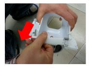
Separate the Flap Lever Rotation Axis from the Ice Shutter and pull it to the direction of the arrow to separate it from the I/SHUT BOX.
