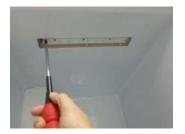
After separating the LED cover, unwind the fixing bolts (2ea) on the LED board.
