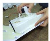
Release the temporary hook of the Louver F A to separate the Motor fixing holes.
