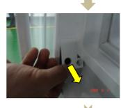
After loosen screw, pull and separate damper cover to arrow direction using a tool.
