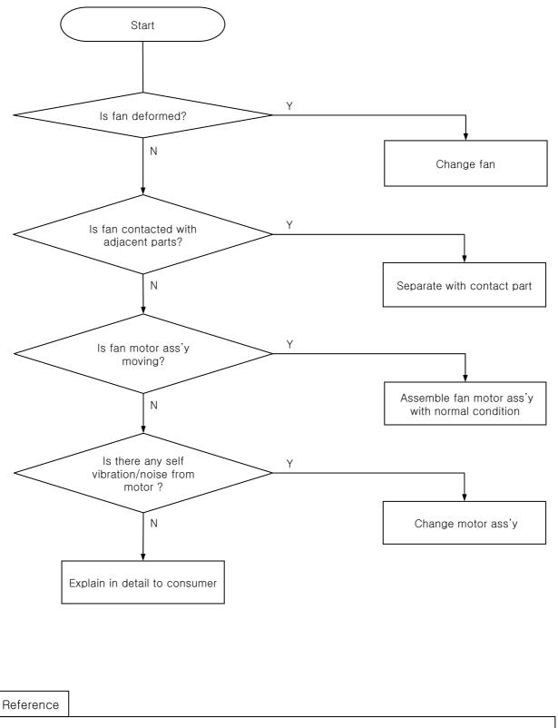
• Noise from louver or wall is in normal condition because wind coming out from fan to make smooth circulation of cooling air inside of refrigerator.
