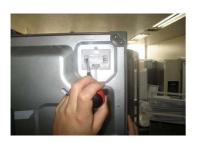
Separate cover & water supply port (silicon rubber) by loosening screw at cover of a water supply pipe at back side of a refrigerator.
