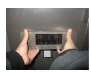
Grip bottom side of a FCB with two hands and lift and pull it forward side to separate FCB.
