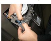
Open up fixing hook and pull out micro switch which is assembled at rear side of a dispenser guide.
