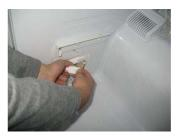
Disconnect harness connected with a damper and pull out a damper.
