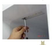
Separate LED cover and loosen 2 fixing screws for LED plate.
