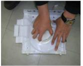
Pull out fan assembled at inner side of a fixture fan motor to vertical direction. [ Fan separation]
