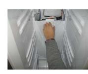
Grip upper part of a duct cover which is assembled at center of a cooler front cover and pull it out to forward direction to separate.
