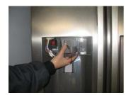
Grip front side of a dispenser guide and separate by pulling it forward.
