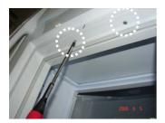
Open home bar door and loosen latch cover fixing screw at upper part of a home bar.
