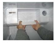
Grip lower side of a damper cover and pull it forward to separate it.
