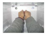
Grip cooling air discharge port at fan cover of a cooler by hand and separate it from lock.
