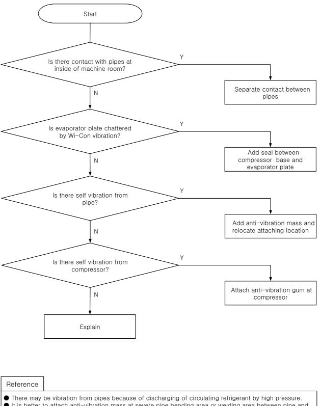
It is better to attach anti-vibration mass at severe pipe bending area or welding area between pipe and compressor when vibration is transmitted to pipe from compressor.
