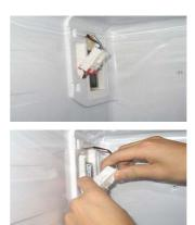
Disconnect harness connected with a damper and pull out a damper.
