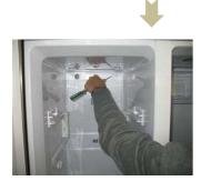
Push back a water supply pipe located at back side of a freezer and go to back side of a refrigerator and pull out a water supply pipe.
