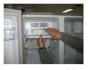
Grip bottom of a ice maker cover and pull it to separate from a freezer.
