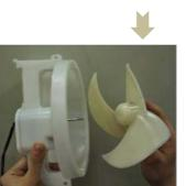
Push and pull forward lock of a bell mouth and separate bell mouth ass'y. (Be careful blade of a fan not to be deformed during disassemble)
