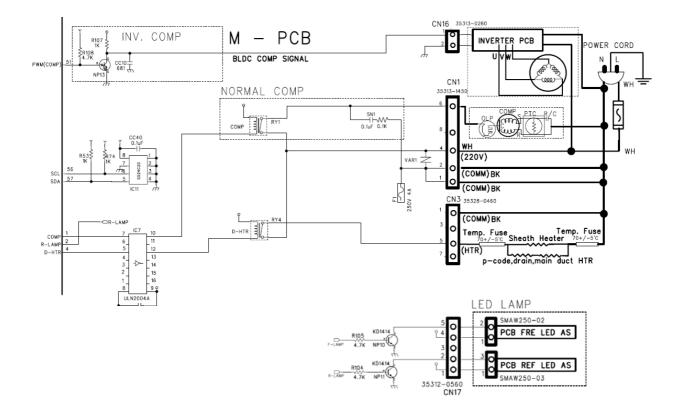
7-3. Relay Operating Circuit & LED Inner lamp Operating Circuit 7-3-1. X22B circuit
