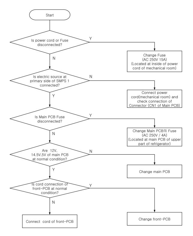
8-1. There is no electric source connected (freezer, refrigerator inner lamp disconnection or F-PCB electric source is dead)
