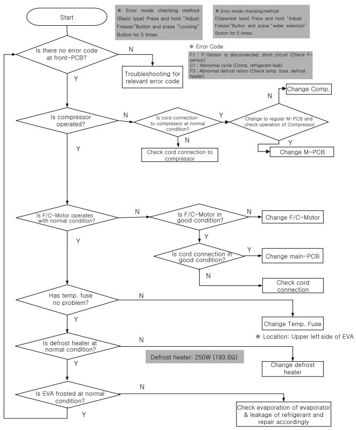
8-2-2. Refrigerator does not operate / Refrigerator is weak in performance.
