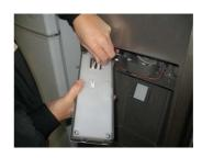
Disconnect 2 harnesses connected with FCB.
