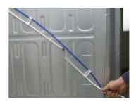
Using check valve, connect water tube. Caution! Check valve is used to protect back flow and connection between tube and assemble so that water supply direction
