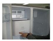
Pull bottom of a ice box and separate ice box from a freezer.
