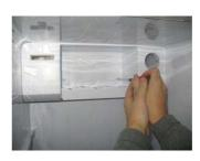
Loosen 2 screws inside of a damper cover.
