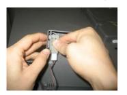
Separate door switch by pressing round shape projected area of a door switch.
