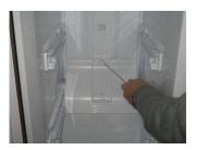
Remove a screw cap at center of a return cover located at bottom of a cooler front cover.
