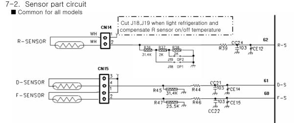
OP1,OP2 : Cut J18,J19 when light refrigeration occur at refrigerator to lower control • temperature of Refrigerator.
