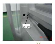
Loosen cover damper fixing screw.
