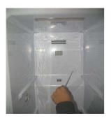
Remove screw cap of a cooler fan located at rear upper side of a freezer.
