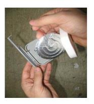
Flap heater can be separated when pull out cushion seal material inside of a flap laver.
