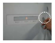
Separate film by inserting (-) driver at right side of a PCB groove at a freezer door.
