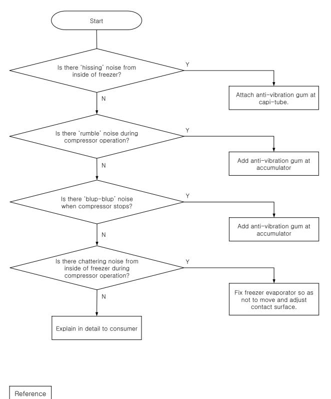
It is at normal operation condition when there is flow noise of refrigerant during compressor operation or "blup-blup" noise when compressor stops because it is refrigerator cycle to change refrigerant from fluid to gas.
