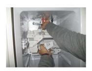
Disconnect harness connected to a ice maker and separate ice maker from a freezer.
