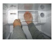
Open window of a damper cover and bend it lightly at center part to separate window.
