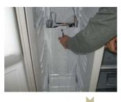
Loosen a fixing screw at cooler front cover.
