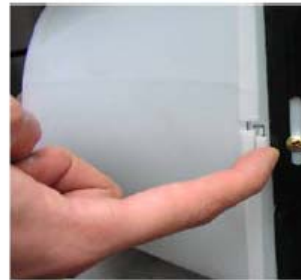
Push and pull forward lock of a bell mouth and separate bell mouth ass'y. (Be careful blade of a fan not to be deformed during disassemble)
