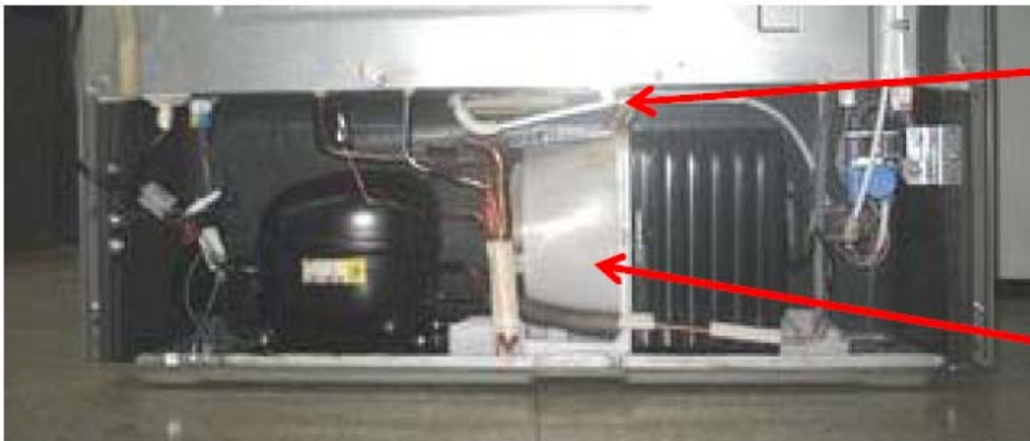
Separate C-fan motor housing at upper right part of a machine room.
