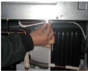
Separate C-fan motor housing at upper right part of a machine room.
