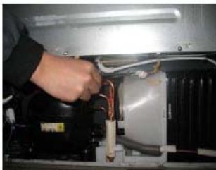
Loosen screws at upper, lower part of a bell mouth.
