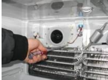
* Remove screws(3ea) of Fixture R Motor B.
