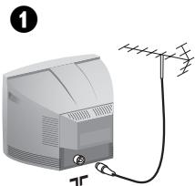
Insert the aerial plug into the **T** socket at the rear of the set.
