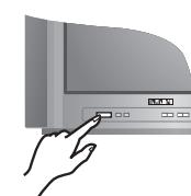
To switch on the set, press the on/off key. If the television remains in standby mode, press **P +** on the remote control.
