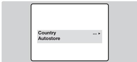
If the menu is not displayed, press and hold down the **◀** and **▶** keys on the TV set for 5 seconds to display the menu.
