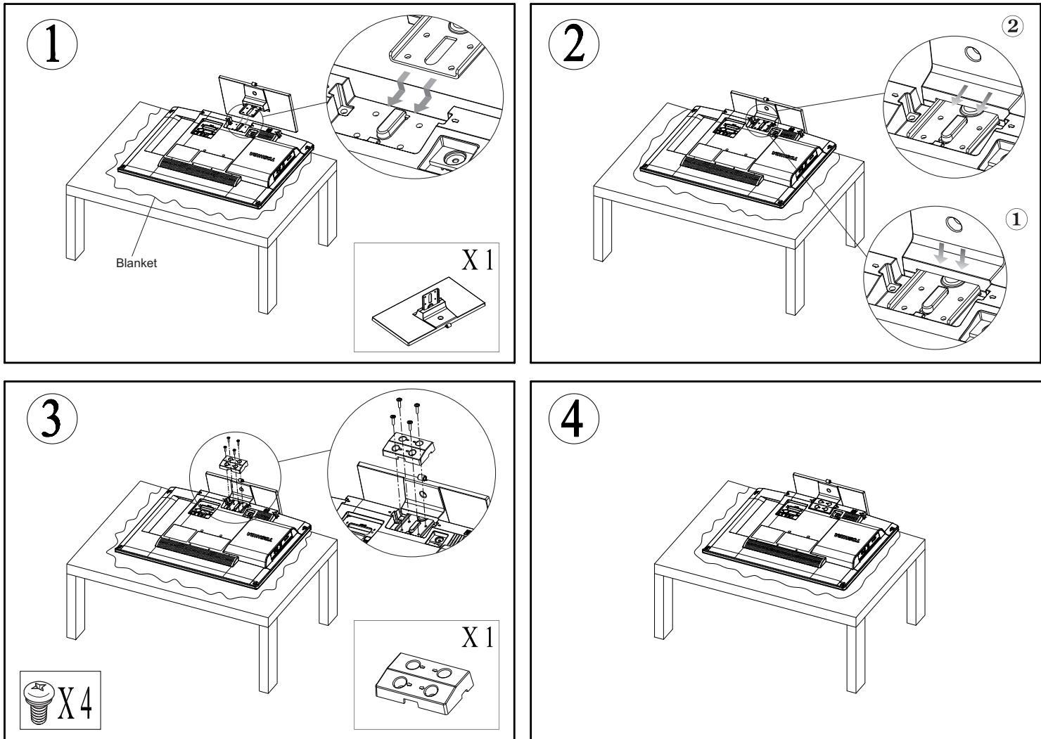
**CAUTION:** Before beginning pedestal assembly, carefully lay the front of the LCD Panel face down on a flat, cushioned surface such as a quilt or blanket. Leave the bottom of the unit protruding over the edge of the surface and assemble as indicated.
