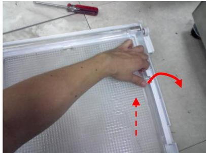
5. Remove the screw and lift up supporter holder
