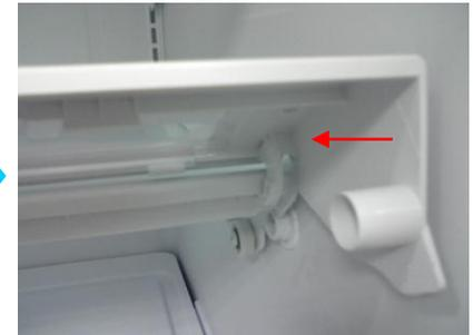
3. Lift and remove the cover assembly tv.
