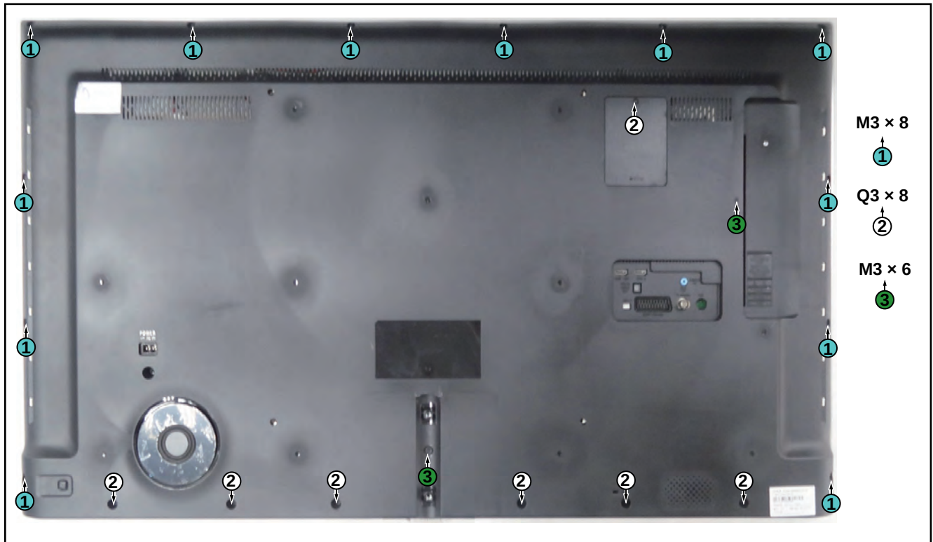
Figure 4-26 Rear cover removal[1]
