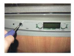
The grey control board housing can now be removed taking care not to pull to far from the fridge as the cable is still attached
