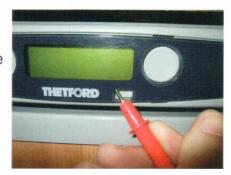
Once the first couple of clips have been released the overlay simply pops out
