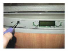
Re-attach the overlay by clipping back in place. The fridge can now be reconnected to the electricity supply and tested
