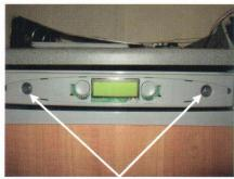
Fully remove the two screws, one found at the bottom of each hole
