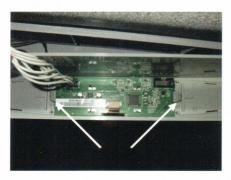
H Simply hold the clips back and remove the display
