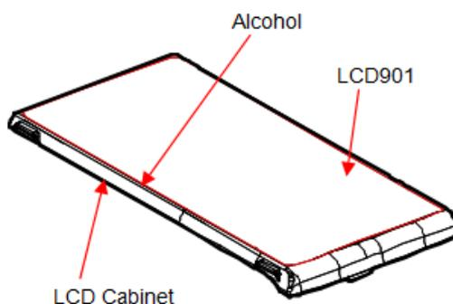
1-2. Remove LCD901 carefully so as not to damage the LCD Cabinet.
