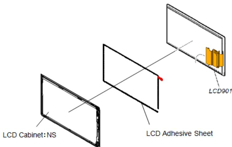
Follow the guidelines below for proper removal / reattachment of "LCD901".
