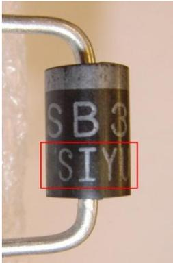
Fig. 3 Dachang source – with “SIYU” marking
