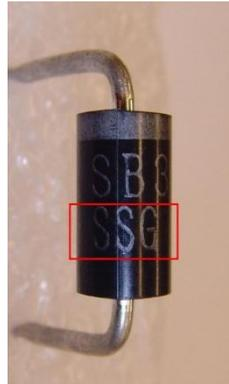
Fig. 4 Sensitron source – with “SSG” marking
