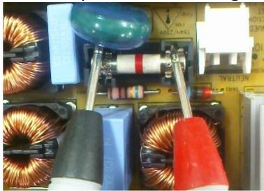
Fig. 9 Fuse F101 measurement
