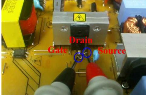
Fig. 7 Q501 Drain-Source measurement
