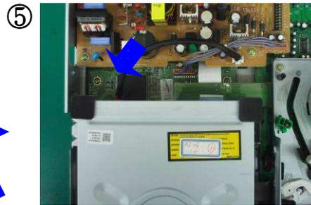
Insert Loader Power cable and Loader assemble
