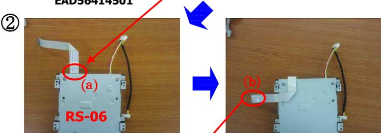
You should assemble EAD56414501 (FFC) and EAD56411801 (Harness) to RS-06 Loader
