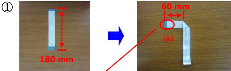
A side of EAD56414501 should be folded. The length is 60 mm.
