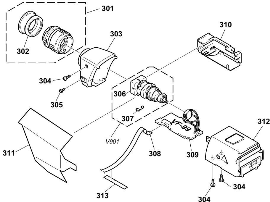
The components identified by mark  $\triangle$  or dotted line with mark  $\triangle$  are critical for safety.
