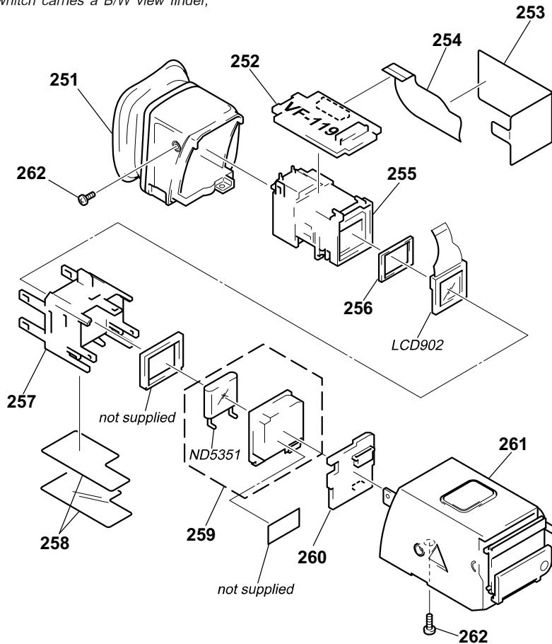
The components identified by mark  $\triangle$  or dotted line with mark  $\triangle$  are critical for safety.
