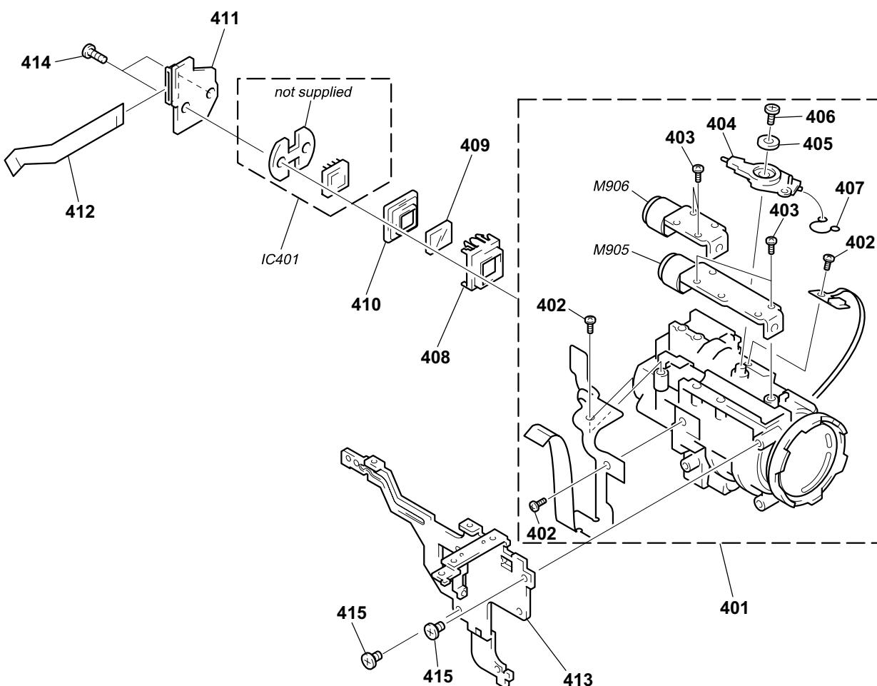
**Be sure to read “Note on the CCD Imager replacement” on page 4-9 when changing the CCD imager.**
