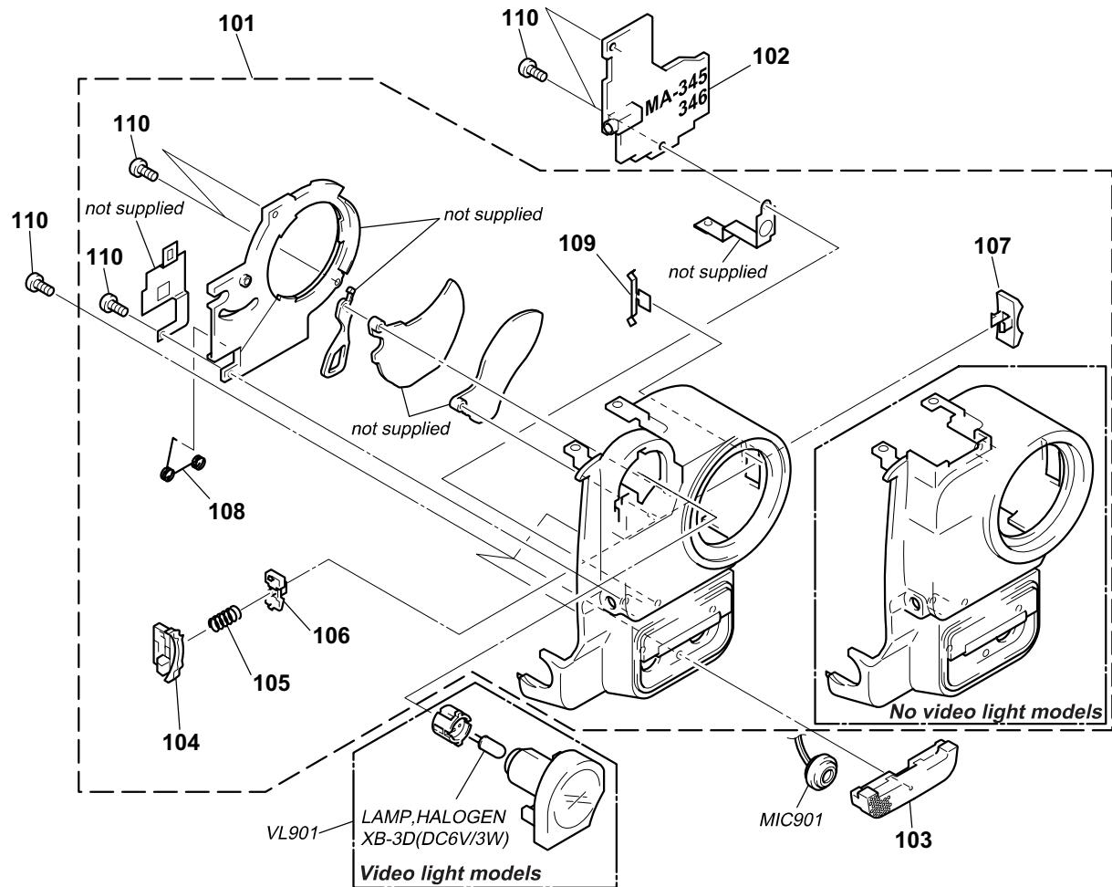
The components identified by mark  $\triangle$  or dotted line with mark  $\triangle$  are critical for safety.
