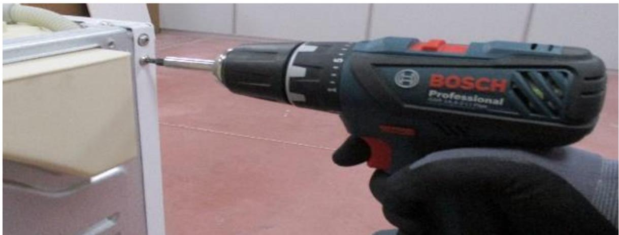
1. To remove the side panels, first remove the 5 screws for each panel at the back.
