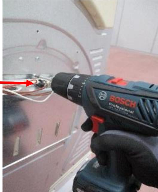
1. Disassemble the heater by removing 3 screws on heater
