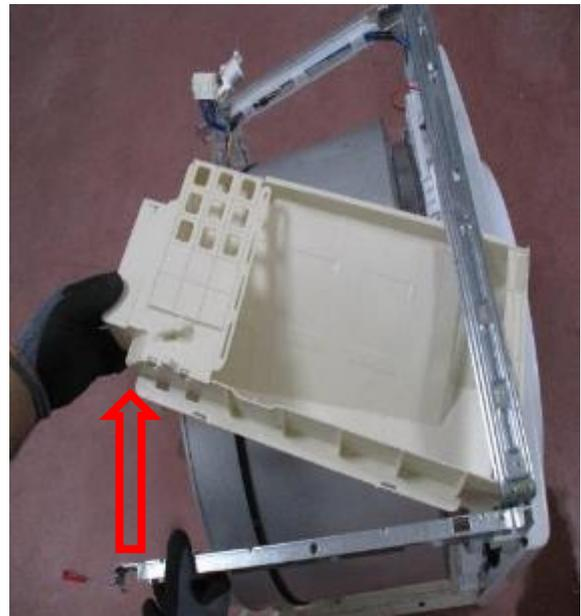
2. Clips fixed to water tank housing with side bracket are removed.
