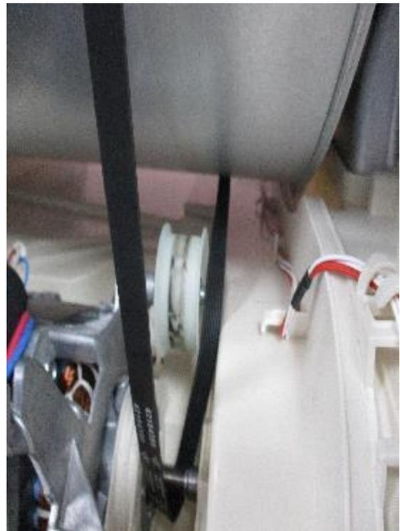
1. Motor should be moved up to prevent to press spring. So, belt will be released as shown in the photo.
