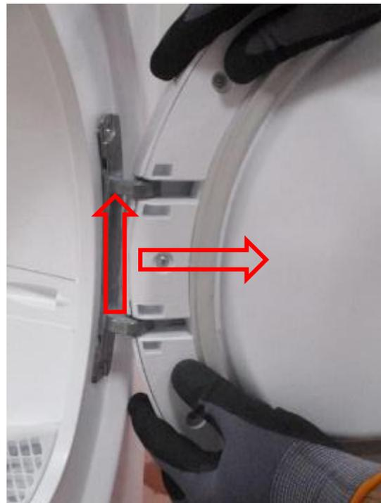
3. Remove two screws on door hinge.
