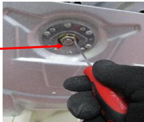
2. Remove the segment on drum shaft.
