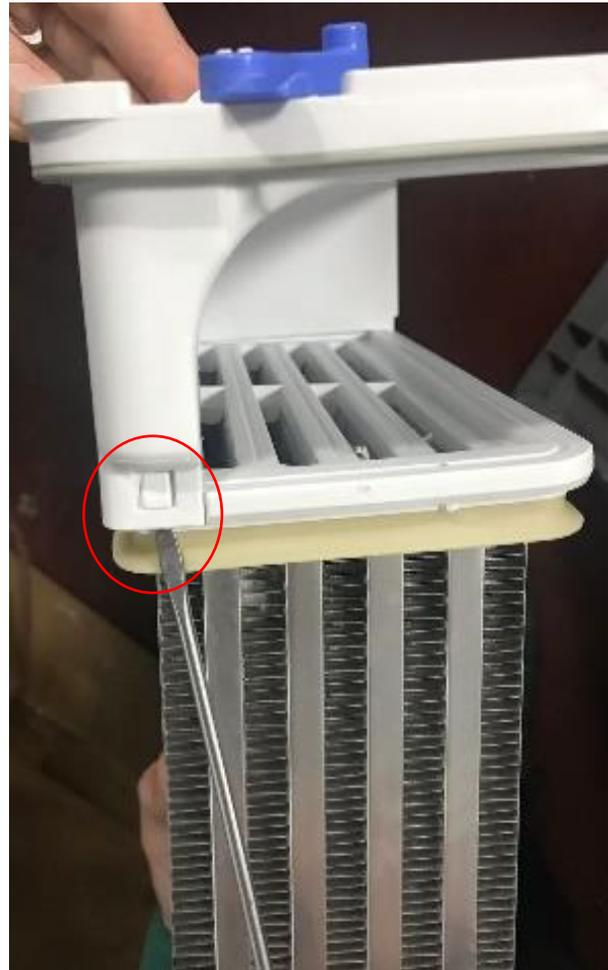
2. The clips around the condenser removed from the slot, as shown in the photo.
