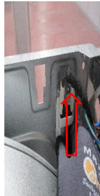
1. There are two heater cable sockets on the outside of the EMI filter, and two power supply sockets (brown left-blue right) on the inside of the EMI filter. They are removed.
