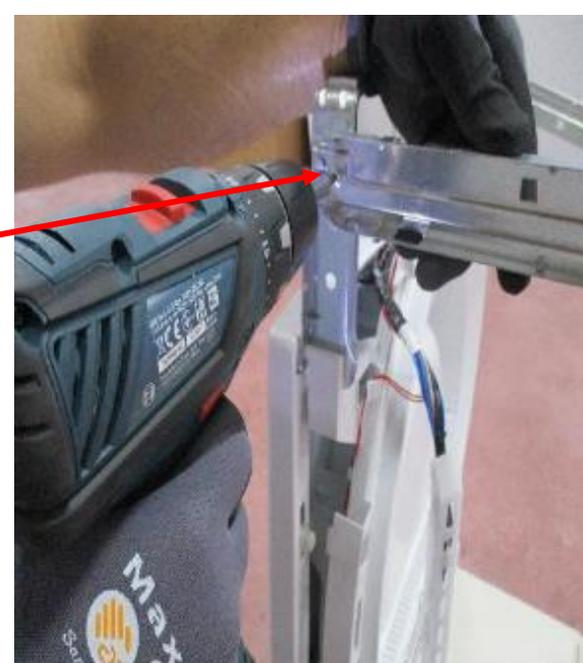
1. Remove the heater cable holder plastic.
