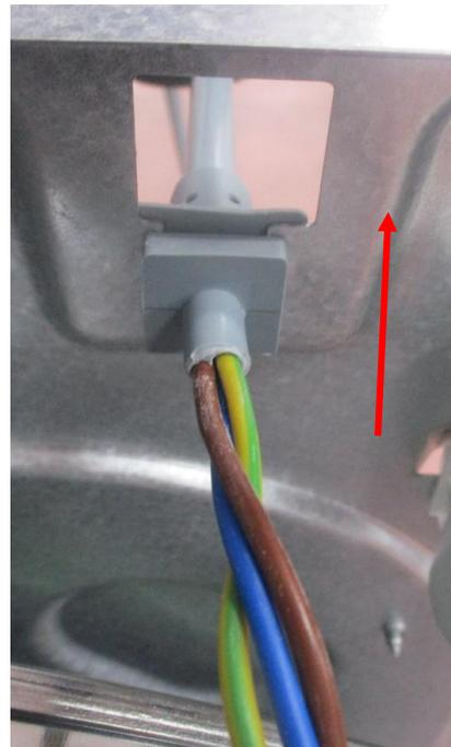
5. Remove the supply cable brown and blue cable socket.
