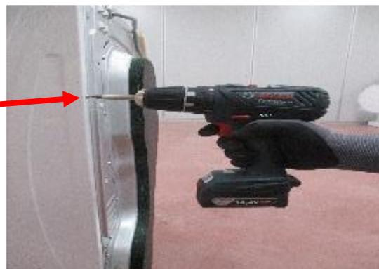
1. Remove all screws on the rear cover shown in the picture.
