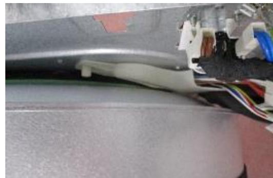
2. In the rear panel, the gasket on the cable group is removed.
