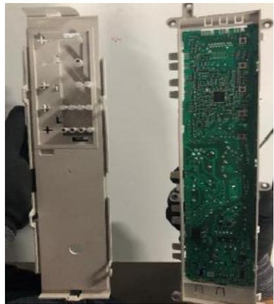
1. For opening the PCB box, press the clips (6 units) Care should be taken not to break the clips here.
