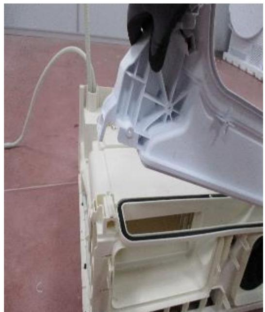
1. Remove two screws fixed of front shield with basement plastic.
