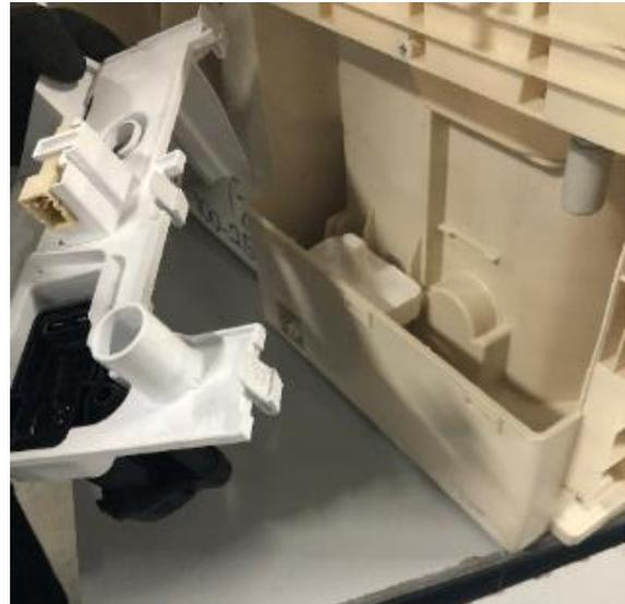
5. Remove 2 hoses that is connected with pump
