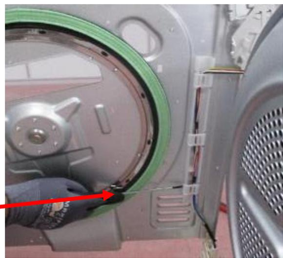
5. Remove the cable group by opening the cable holder plastic canal.
