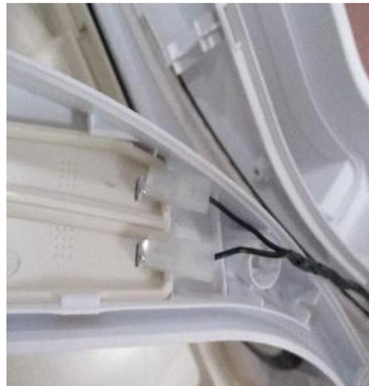
1. Screws of humidity sensor plastic are removed.
