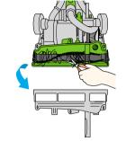
Clear the brushbar obstruction. Carefully cut away any threads from the brushbar.
