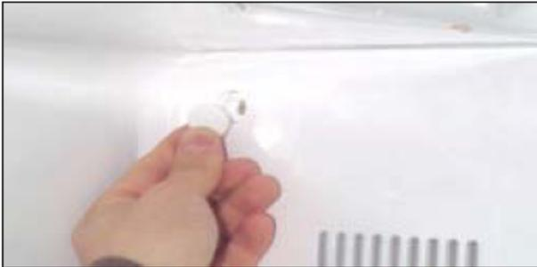
1) Remove screw cap on the Freezer Louver.
