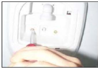
3) Unscrew which fixing the control box.
