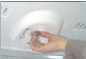
2) Disassemble refrigerator lamp.
