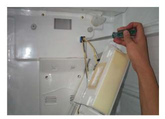
6) After romoving the control switch knob and two screws for fixing control switch, change the control switch to new one.
