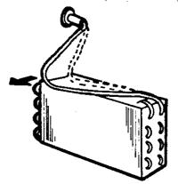
3) Move the entire eveporator upward the pipe center to the arrow's direction.(Do not crumble the part A of the accumulator during the process.)
