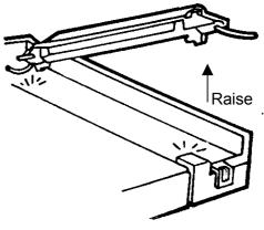
5) Pull out the glass tube heater from the heate supporter with heater covers remaining.(upper and lower) (Do not apply much power on the heater supporter.)
