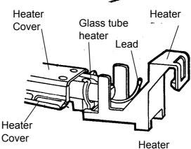
6) Install the heater covers (upper and lower) on a new glass tube heater. (Make the cover with holes the lower one)
