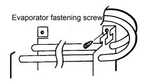
2) Slightly pull the evaporator to the arrow's direction.
