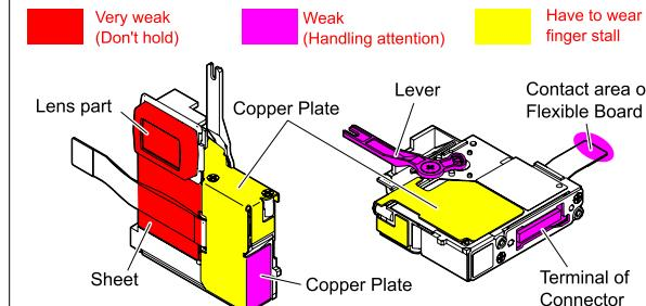
The projector unit (copper plate in particular) becomes hot after it is used. When replacing a part of the projector unit, wait until it is cooled down.
