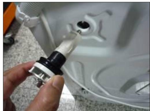
2. Hold the tub bellows seal and gasket-body fixing spring together, and pull them up.
