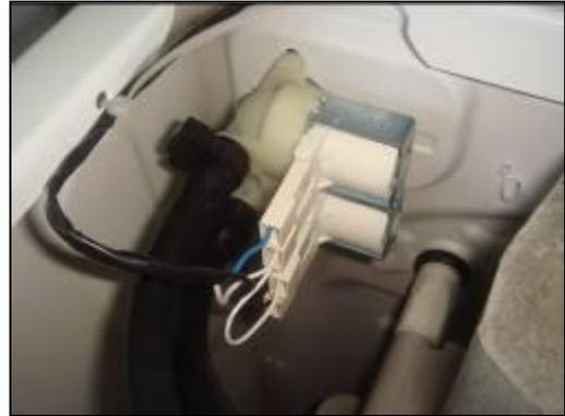
3. Turn the feed valve counter clockwise slightly to remove.
