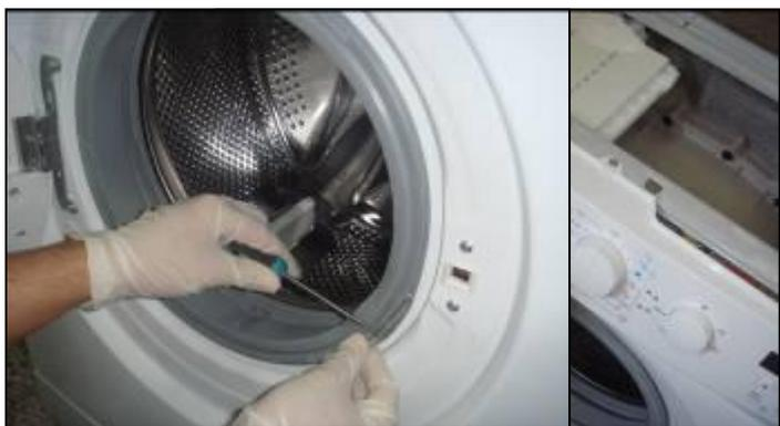
2. Remove the tub bellows seal-body fixing spring.
