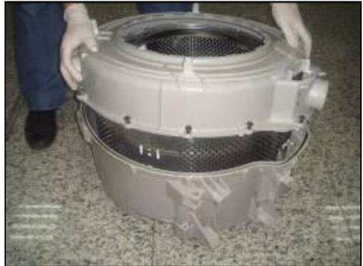
2. Remove the tub exit with bellow hose with ball by using box wrench size 10 mm.
