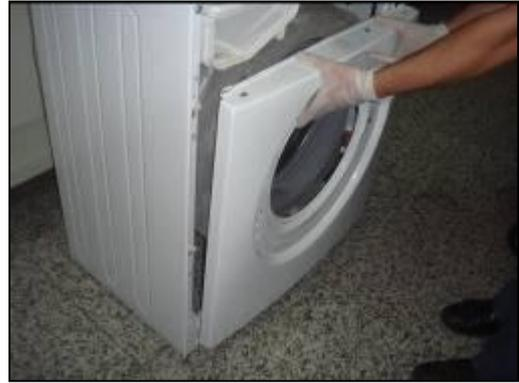
5. Remove two screws fixing front panel at the below as it is shown in the picture.
