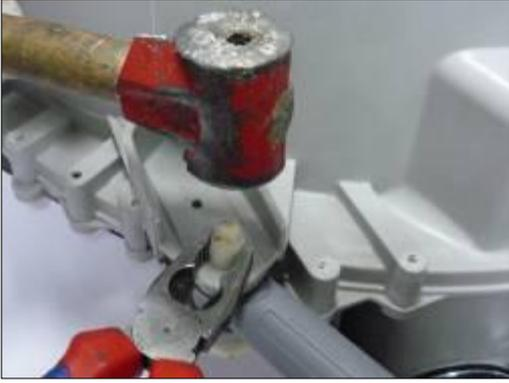
2. Remove the driven pulley it is shown the picture.
