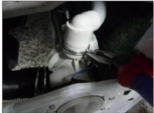
2. Remove pipe clip fixing the tub outlet hose.
