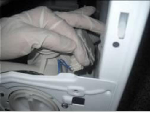
4. Remove four screws fixing the pump motor.
