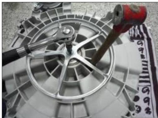
2. Pull the motor up for disassembly.
