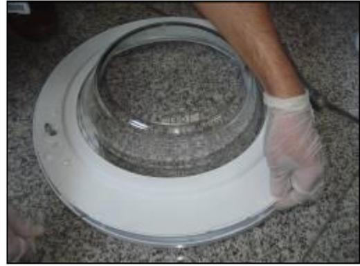
5. Remove the door inside plastic as it is shown in the picture.
