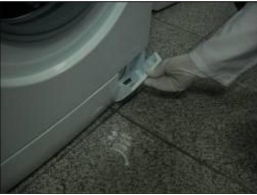
2. Remove two screws fixing the kickplate.
