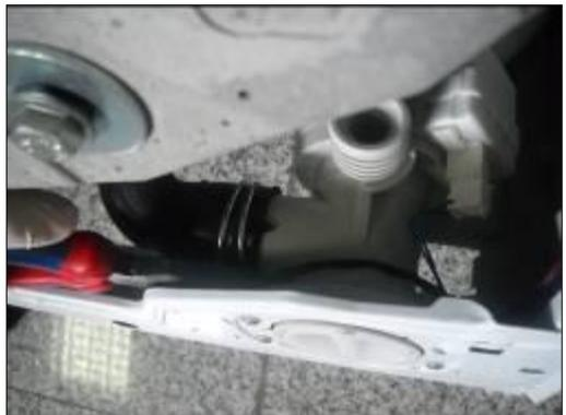
3. Remove the connector that is connected to the pump motor.
