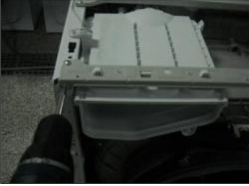
2. Remove two screws fixing the body group at the upper as it is shown in the picture.
