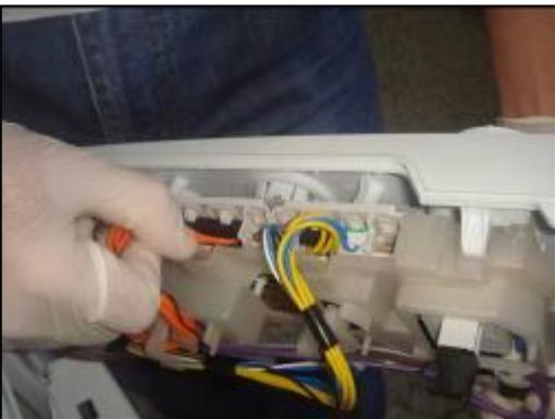
5. Remove the lcd communication cable as it is shown in the picture.
