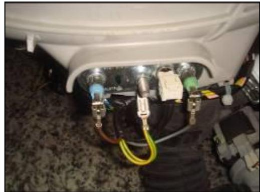
2. Remove one nut fixing the heater slightly (box wrench size 8 mm)
