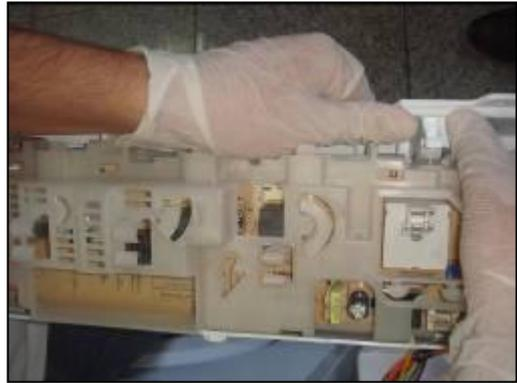
7. Remove lcd electronic card as it is shown in the picture.
