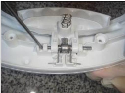
8. Remove the door handle pin as it is shown in the picture.
