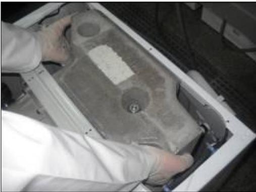
3. Remove the four screws fixing the spring hanger sheet iron.
