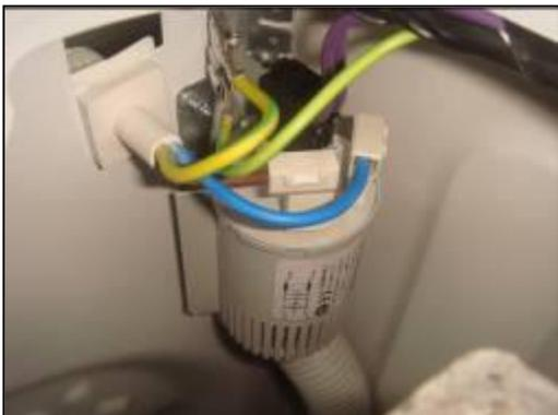
2. Remove two screws fixing the parasite filter.
