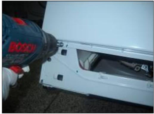
2. Remove two screws fixing the door lock as it is shown in the pictures.
