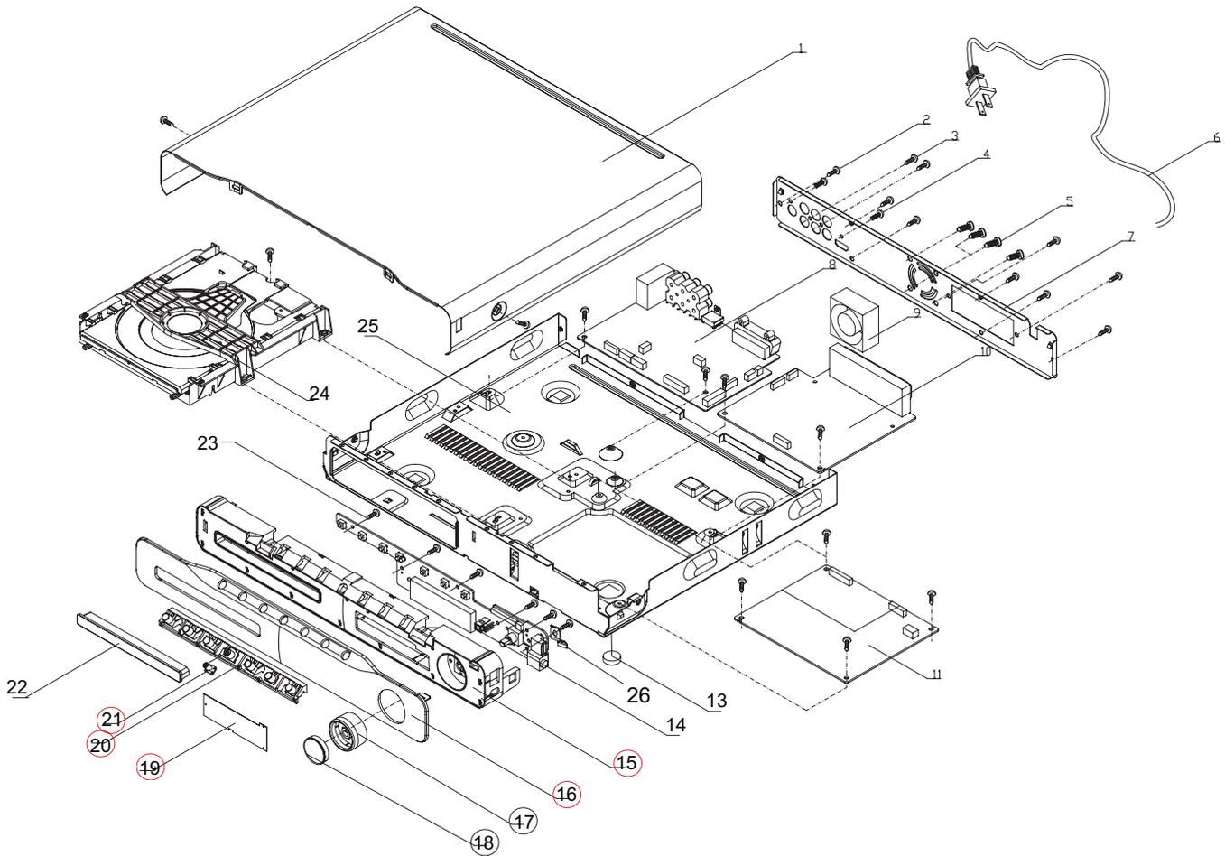
It is general mechanical exploded view for HTS3520/51/X78/94, detailed information pls refer to the model set.
