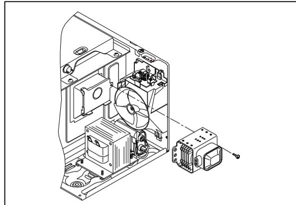
**CAUTION** : Never install the magnetron without the metallic gasket plate which is packed with each magnetron to prevent microwave leakage. Whenever repair work is carried out on magnetron, check the microwave leakage. It shall not exceed  $4\text{mW}/\text{cm}^2$  for a fully assembled oven with door normally closed.
