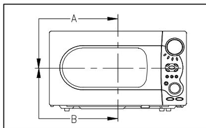
**NOTE :** A small gap may be acceptable if the microwave leakage does not exceed 4mW does not exceed 4mW/cm<sup>2</sup>.
