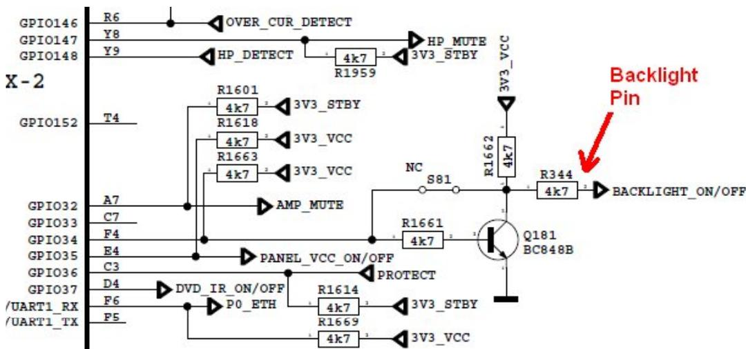
Dimming pin should be high or square wave in open position. If it is low, please check S16 for Mstar side and panel or power cables, connectors.
