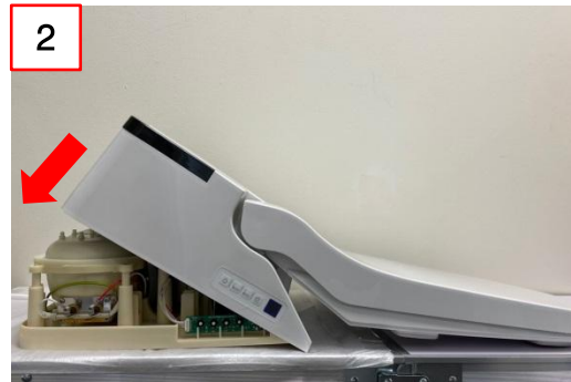
② Close the cover base in the direction of the arrow.
