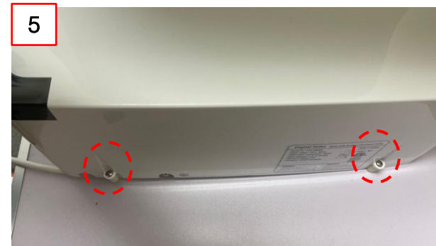
⑤ Tighten screw 2EA using a driver.
