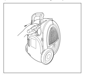
3) Disassemble the body cover, raising the body cover.
