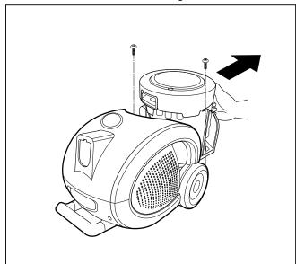
2) Remove the four screws fastening the body base.
