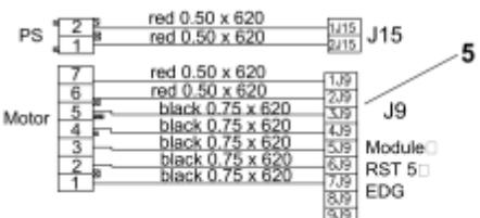
WIRING N = MOTOR + PUMP COD. C00093719
