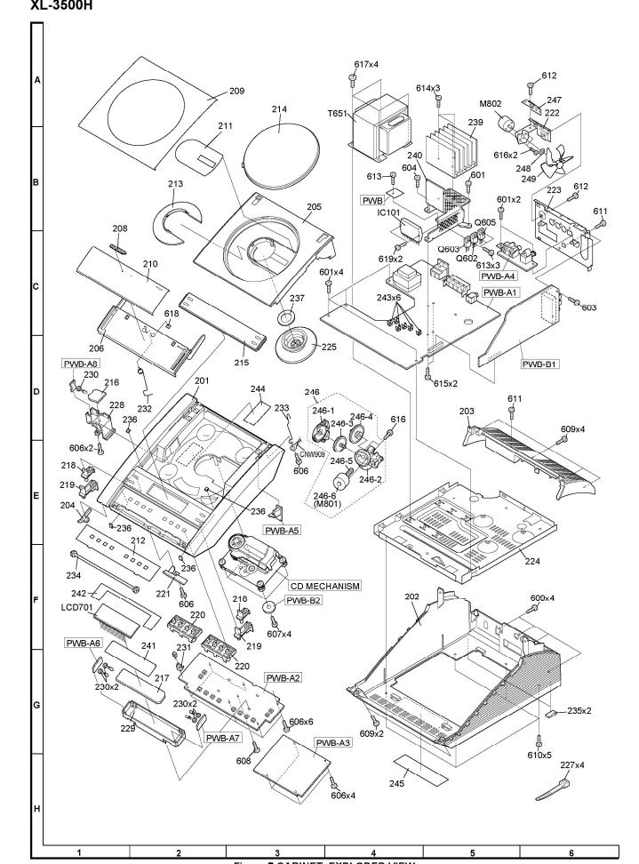
Figure 7 CABINET EXPLODED VIEW
